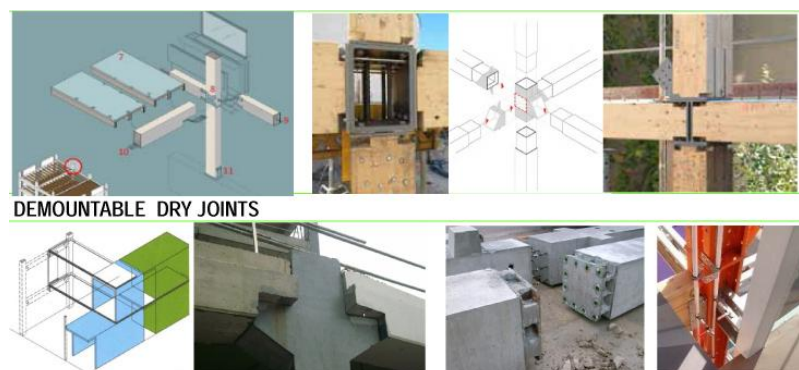
Fig.12: Demountable dry joint in load-bearing structure
