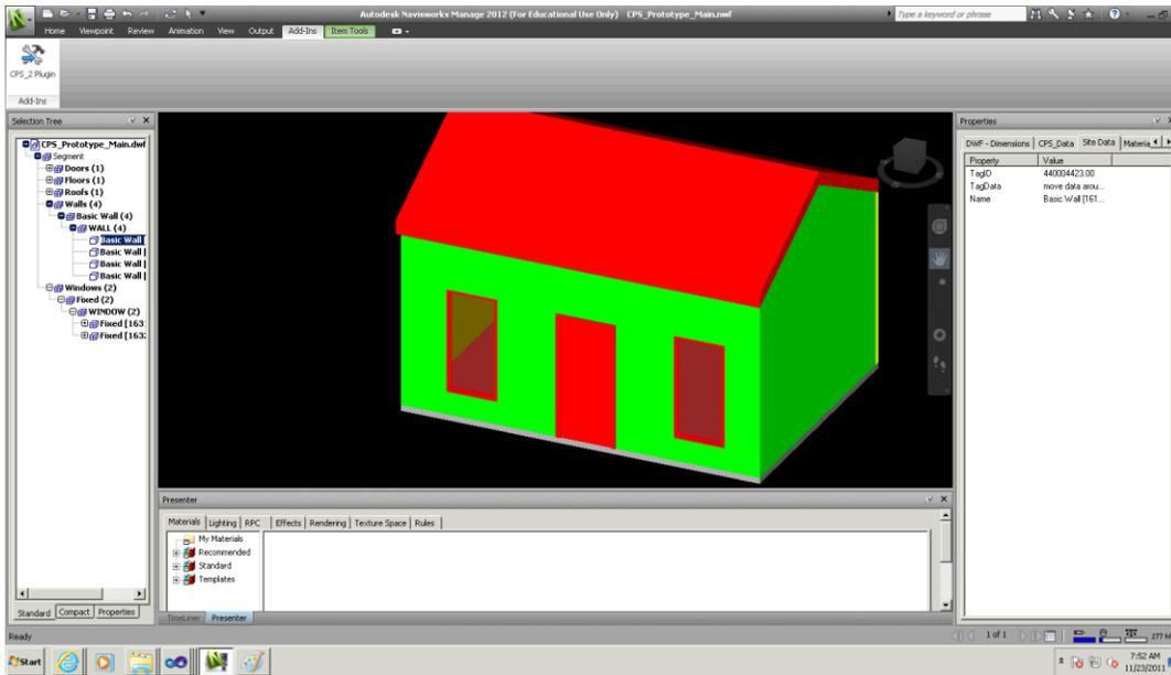
Figure 6: Door and Roof element status changed to 'uninstalled' (red)
