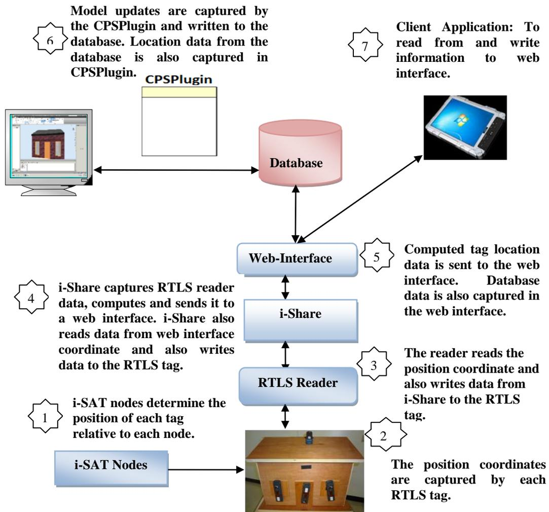
Figure 5: Overview of Prototype System
